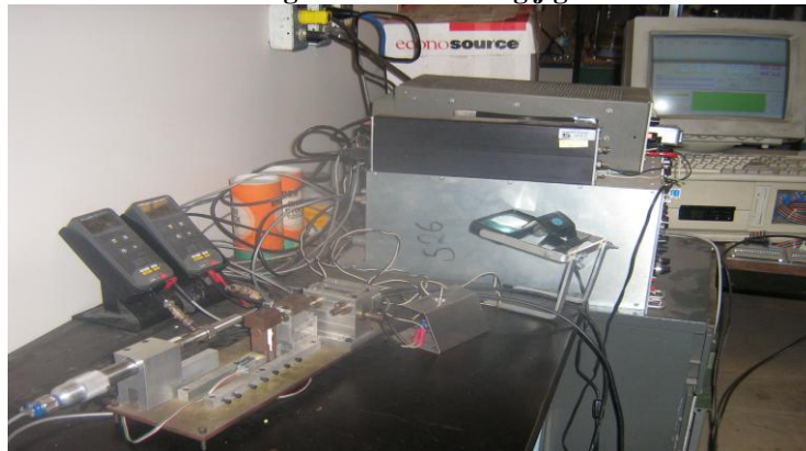
Figure 5 Fibre testing jig setup with computer for data recording
